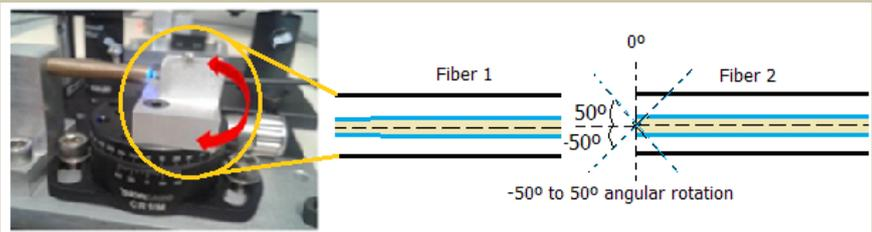
Fig. 2. Experimental system of angular position fiber sensor.
